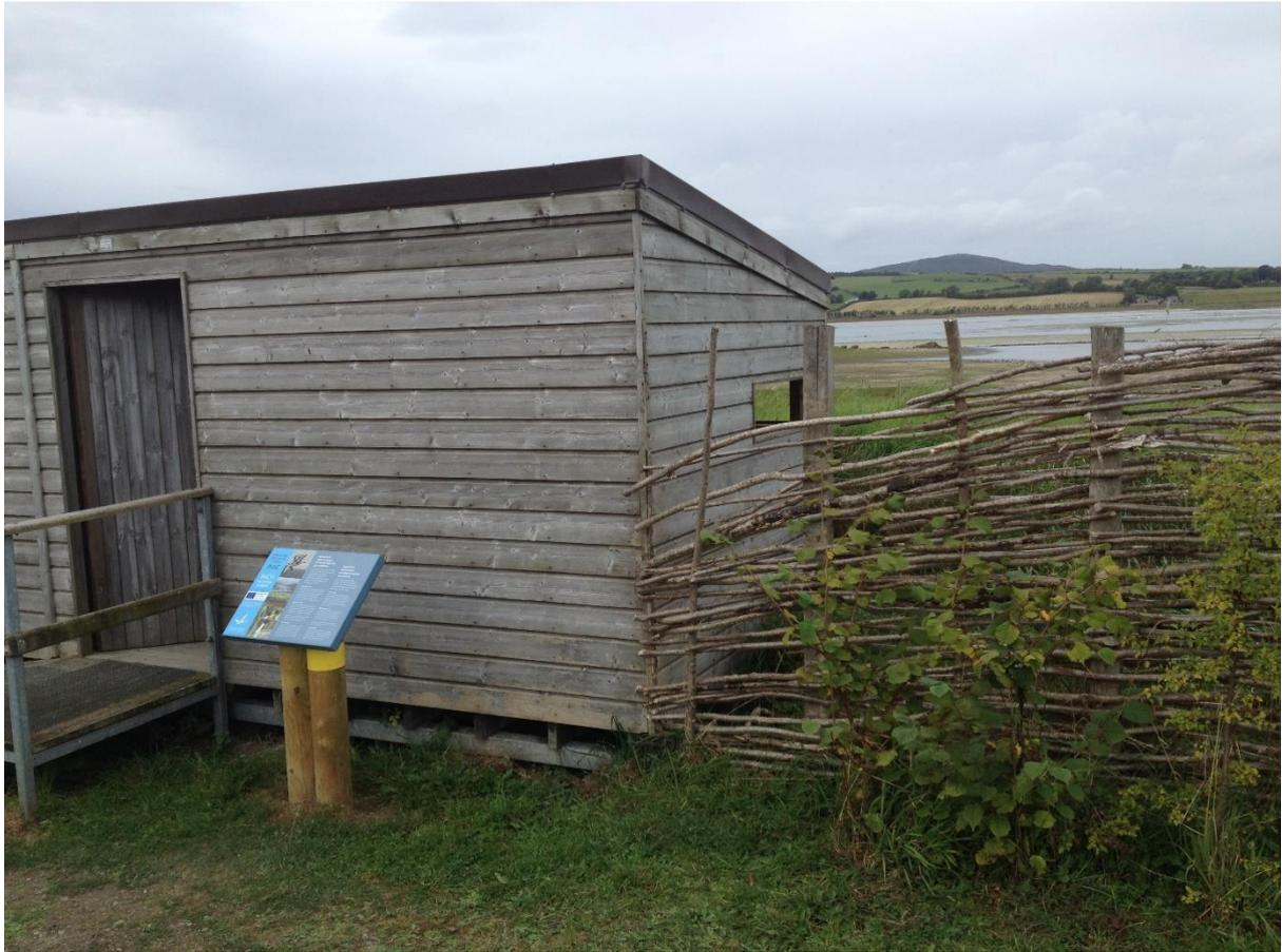
This birdwatching hide is well screened to each side using a woven hazel panel which helps to boost the screening provided by natural vegetation growth. The screen here needs some maintenance to be fully effective!
